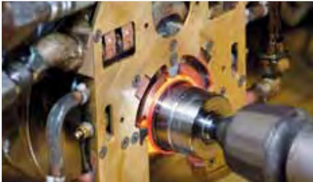
The area to be hardened is heated up by the inductor and quenched in just a few seconds.
