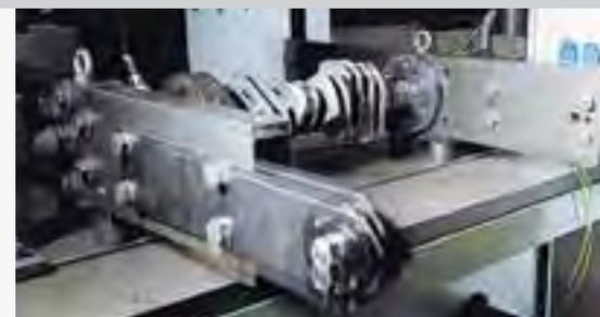
A torsion test bench developed by the company determines the torsional fatigue strength of an automotive crankshaft using programmable automated test procedures.
