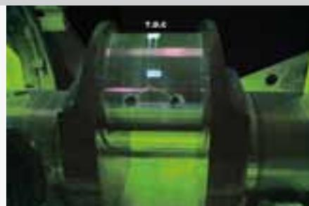
A torsional fatigue strength test resulted in a crack in the pin journal: the root cause analysis is about to start.
