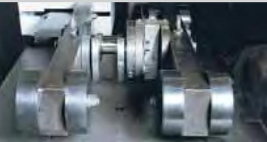
**Test rig for determining the alternating bending and torsional fatigue strength of a crankpin.**
