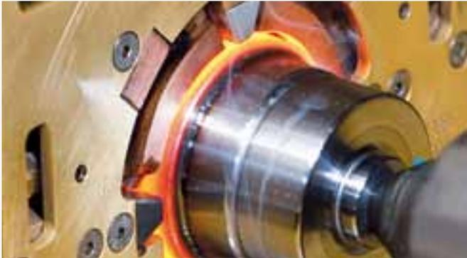
**Optimal interaction between inductors and frequency converters ensures the shortest possible heating times.**
