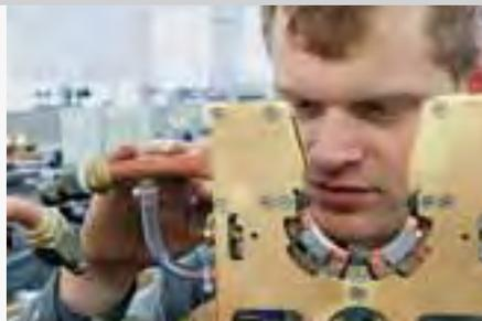
**Final assembly and adjustment of an inductor.**
