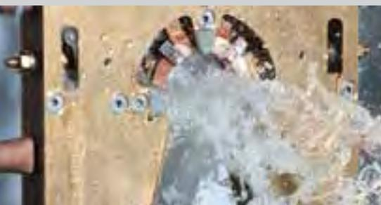
Comprehensive testing series using different inductors and quenching media can be performed on a specially installed hardening machine in our application center.
