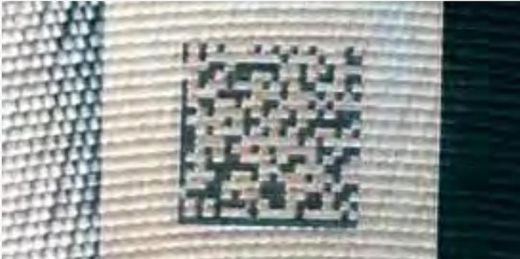
Production data can be marked on each crankshaft, e.g. via data-matrix code. This makes it possible, besides the production data, to analyse the hardening results for retraceability.
