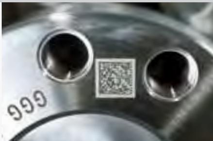
**Automatic reading of the data-matrix code ensures a reliable identification of the workpiece.**
