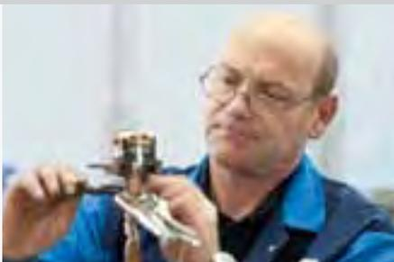
**Assembly of the delicate heating coil of an inductor.**
