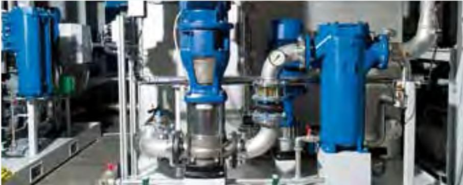
Standardised recirculation cooling units are used for cooling the quenching media, inductors and other electrical components.
