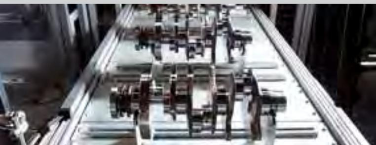
**Loading and unloading conveyors ensure a reliable material flow.**
