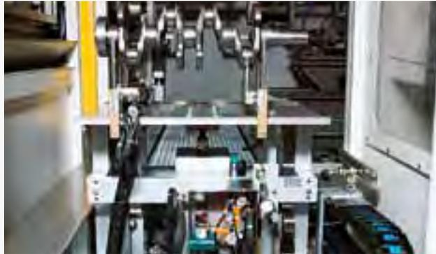
Production processes are only efficient if the hardening system is an integral part of the customer's production line. Therefore we offer a variety of conveyor systems which can be individually configured. We ensure harmonisation of all interfaces around the core process of induction hardening. We can supply automatic conveyor systems as well as systems for safe manual handling of the workpiece loading and
