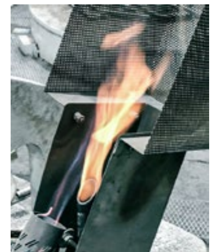
FLARING OF PROCESS GAS AT HARDENING SHOP
